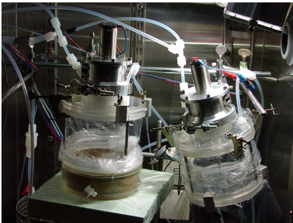
Figure 2.2: Reference cuvette (right) and soil sample cuvette (left), all built of Teflon, incubated in a climate chamber.
