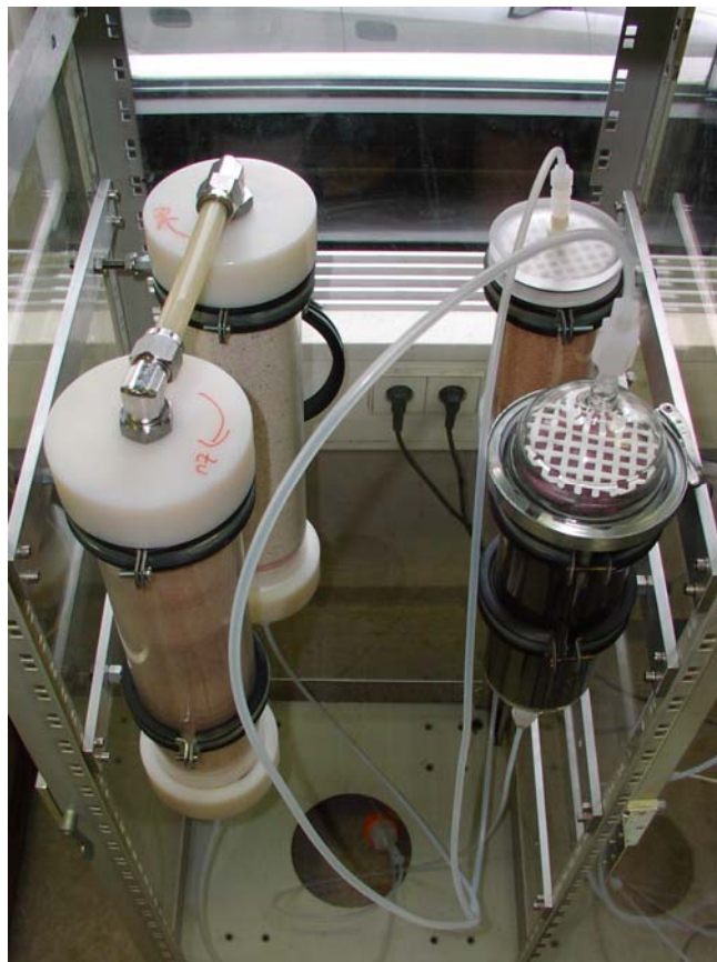
Figure 2.1: Purification system with four Plexiglas-columns filled with (2 times) silicagel, molecular Sieve and charcoal.
