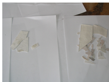
(a) Separation of old, used LiF parts with and w/o glue and removal of glue with scalpel.
