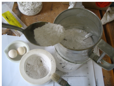
(c) After the mill the powder is sieved to filter out unseen pieces of glue.
