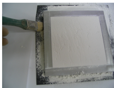
(f) Use brush to remove the LiF from top the frame and around the frame and recollect the powder.
