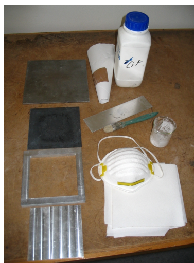
(d) Required material: steel plate (5 mm thick, 18 \times 18 \text{ cm}^2 ), funnel, container for LiF powder left over, thin plate, brush, Al-plate, Al-frame (11 mm thick, 11 \times 11 \text{ cm}^2 ) + Al-plate that fits in, breathing protection, AlO-foil (3 pieces, each 12 \times 12 \text{ cm}^2 ).
