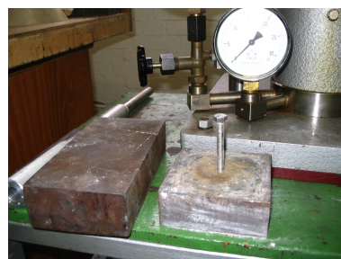
(b) The fitting AL-plate has to be placed on the powder inside the frame (w/o picture). A steel brick with the same dimensions comes on top and can be hold be a screw.
