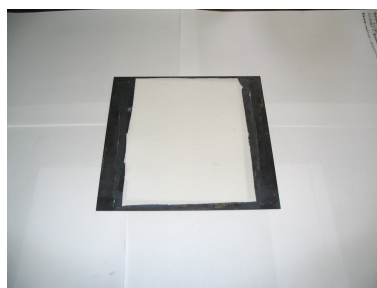
(f) Cover it with two pieces of AlO-foil which prevents the LiF to react with the steel surface while baking.
