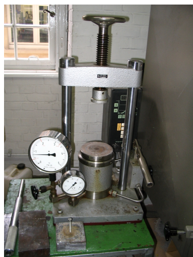
(a) The hydraulic press is used to solidify the powder into a \approx 5 cm thick plate.
