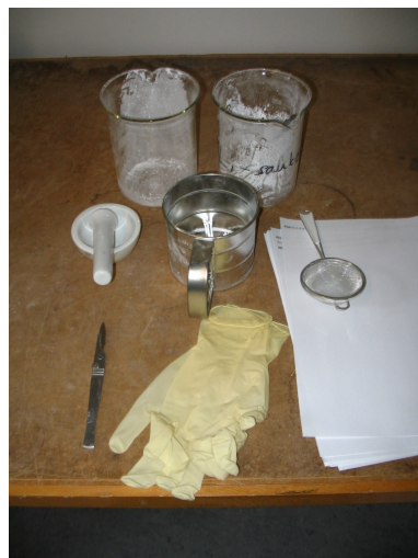
(a) Required material for cleaning: 2 beakers (1 for crushed LiF, 1 for powder), mortar, 1-2 sieves (raw/ fine), scalpel, gloves, paper.
