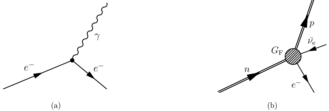
Figure 2.1: Feynman graphs: (a) An electron-photon vertex. (b) Neutron decay in Fermi's presentation. The time arrow is pointing to the right.
