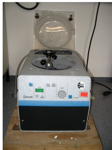
(b) A mill (type “Retsch S1000”) is needed to make powder out of the pieces. Duration: 45 min at “Speed=70”.
