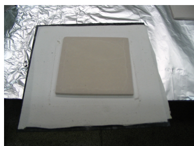
(e) After backing. Sometimes the edges may brake.
