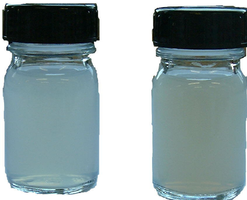
Figure 58 Inverse micelles solutions: PS 192 - b -hypPG 110 (left) and linPG 24 - b -PS 192 - b -linPG 24 (right).
