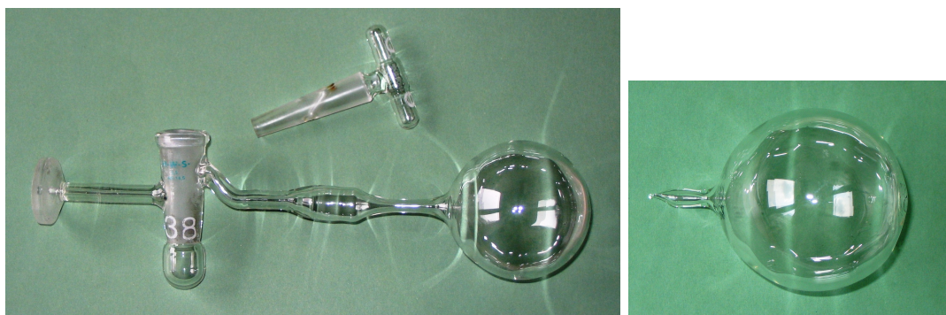
Figure 3.3: Magnetometer cell out of GE 180 glass with appendix and stopcock ( left ) and filled with ^3\text{He} after the sealing ( right )
