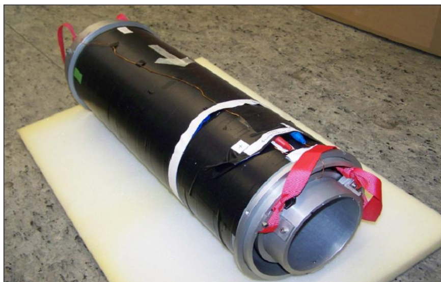
Figure 4.4: Transport coil for the transfer of the polarized gas from the filling station to the shielded cabin.
