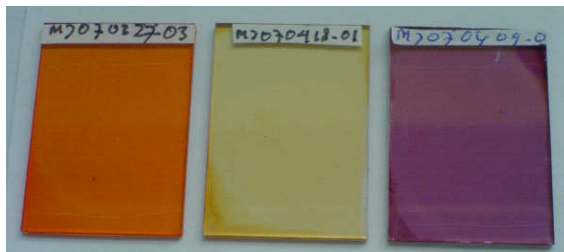
Fig. 5.4: Photographs of very thin ( d=50-70 nm) films of P3HT: regiorandom (left), regioregular (right) and blend of 10% regioregular and 90 % regiorandom (centre).
