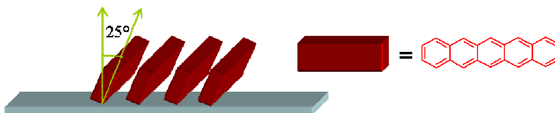
Figure 98. Schematic view of the PEN arrangement on the glass surface.
