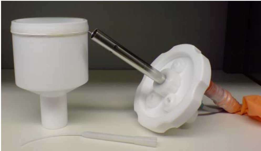
Figure 5.14 Conductivity vessel, completely made out of PTFE, Probe made out of steel.
