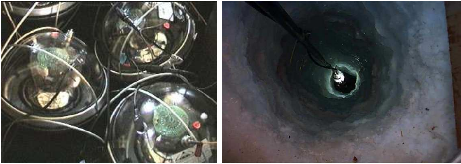
Figure 2.9: Left: AMANDA optical modules, composed by a photomultiplier enclosed in a glass sphere. Right: Deployment of a string in ice seen from the surface.
