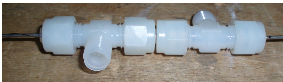
Figure 2.13: A completed enrichment trap with housing.
