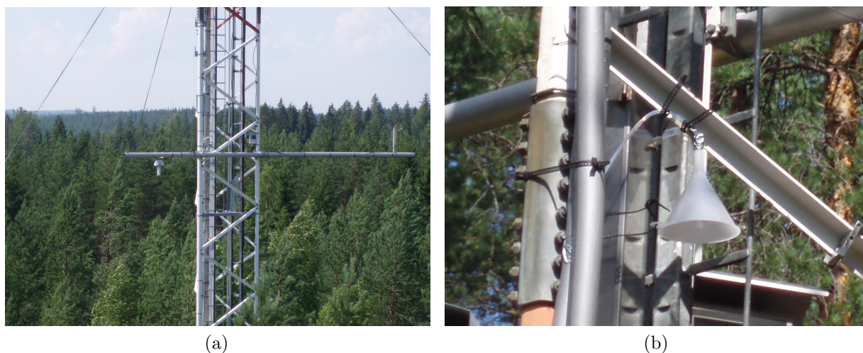
Figure 4.3: Sampling inlets during the HUMPPA campaign: (a) showing inlet height for FOTOS with respect to canopy (the inlet was level with the long horizontal bar shown) and (b) showing the methane inlet with filter and rain shield from below.
