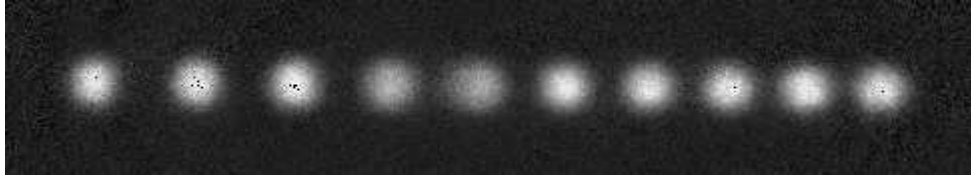
Figure 1.14: All Zeeman components of ^{40}\text{K} atoms revealed in a Stern-Gerlach experiment during time of flight.
