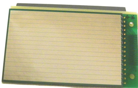
Figure 2.3: Photograph of a DSSD, which can be installed behind the exit window in the focal plane of TASCA.
