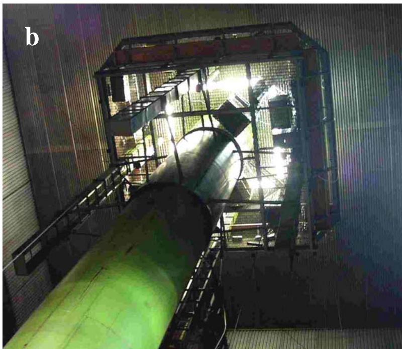
Figure 5.2. Fire Sciences Laboratory (a) fuel bed and inverted-funnel exhaust stack (b) sampling platform (at 17 m height).
