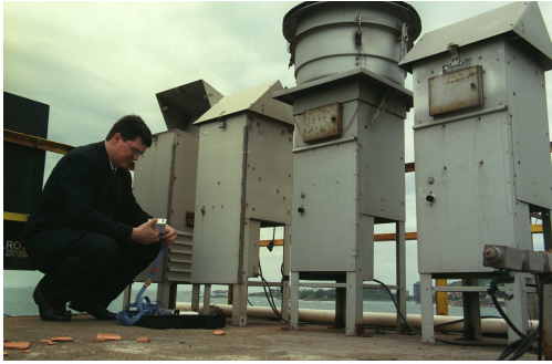
Figure 5.1: Air pollution samplers located at Ilha do Boi, Vitória, Brazil.
