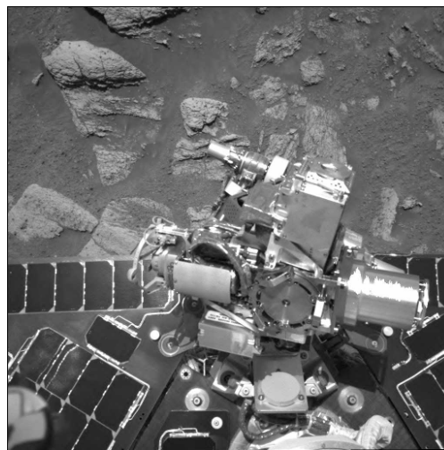
Figure 3.7: The region called "Last Chance" can be seen in the background at upper left in this navcam image. In the foreground, Opportunity examines its tool turret. The "wrist" of its robotic arm is behind the turret. The rock abrasion tool is pointed to the left; MIMOS II is pointing upward in the image. The alpha particle X-ray spectrometer is pointing to the right.
