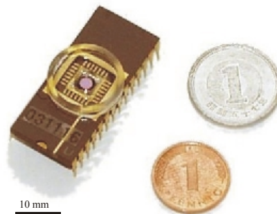
Figure 3.20: Photo of an EOSFET array chip mounted onto a DIL ceramic carrier. The chip contacts were sealed by a silicon funnel surrounded by a glass ring, which served as a container for the electrolyte bath.
