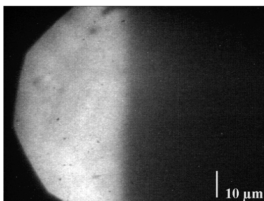
Figure 5.23: Monolayer edge of DSPC on Chitosan, lateral transfer pressure 40 mN/m.
