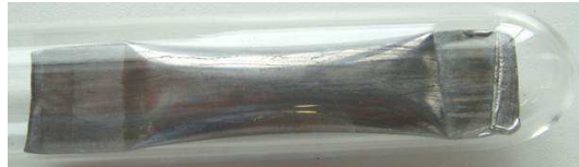
Figure 10.11: Sealed tantalum tube in quartz tube used for the synthesis of LiZnP.
