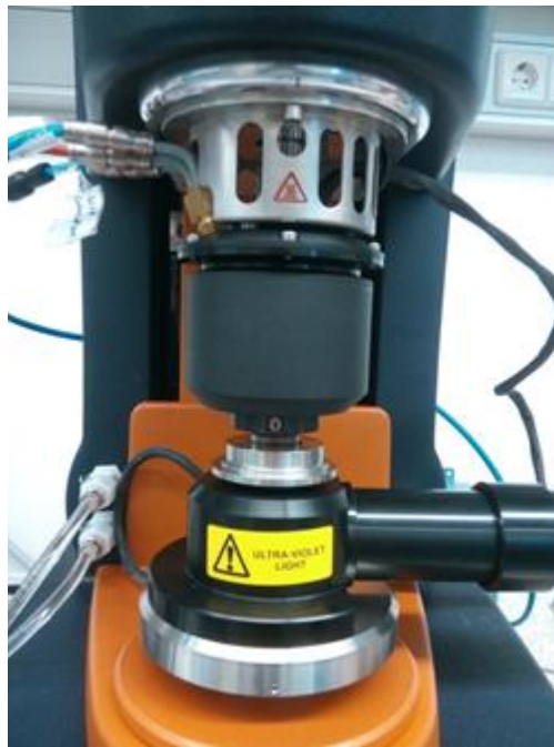
Figure 1.17 Photograph of TA-DHR3 rheometer with upper-heating plate for temperature control and UV curing plate.
