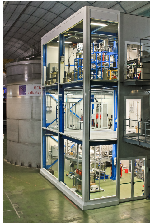
Figure 7.1 – Picture from the XENON1T experiment in the hall B of the LNGS. The foreground shows the support building where the ReStoX, xenon purification system and further electronic is mounted. In the background, there is the XENON1T water tank shown [44].
