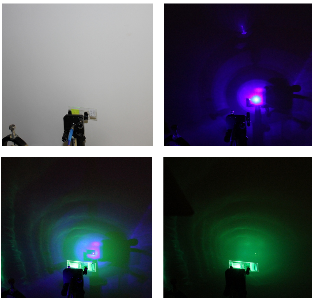
Figure 3.52: Interference rings and fringes of a YP doped cellulosic CLC film above threshold. The sample under white light (top, left), the excitation pulse without sample (top, right), the sample under excitation (bottom, left) and the same situation using a filter to remove the pump light.
