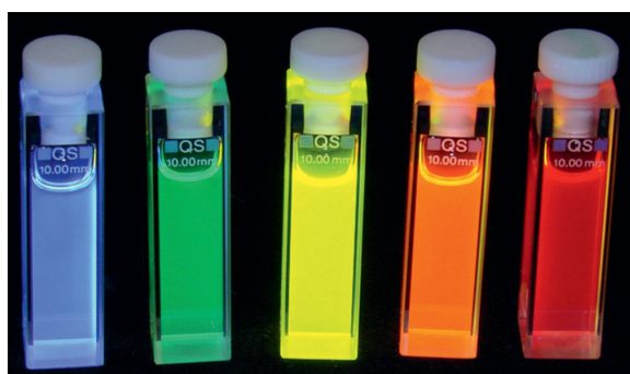
Figure 1.21: Fluorescent semiconductor nanoparticles in solution. The emission wavelength is dependent on the particle size (increases from left to right) [126].
