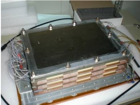
Figure 2.9: Photograph of BDC (Beam Drift Chamber)
