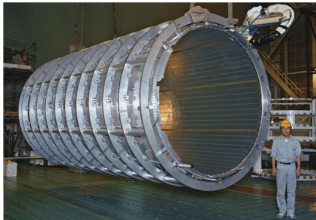
Figure 3.18: The ATLAS solenoid magnet [61].
