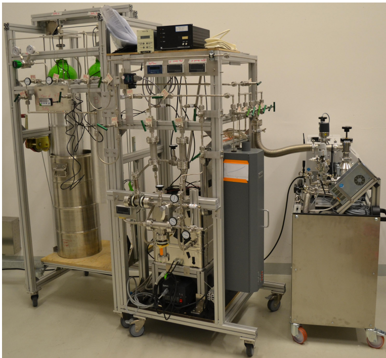
Figure 3.9: The gas system is the large structure on the lefthand side, which can be seen as two connected parts. The left is the holding structure for the xenon bottles with two bottles (colored in green) connected. They can be seen hanging from the structure, with the left one being partly inserted to a dewar for liquid nitrogen. This is for the cryopumping during the recuperation process. The right part of the gas system is the recirculation part, including the gas purifier in the grey box and the pump in the metal box in the lower center of the picture. The flowmeter as well as displays for pressure sensors are installed at eye height. The device on the right is a pumping station which is evacuating and therefore cleaning the gas system before operating with xenon gas.
