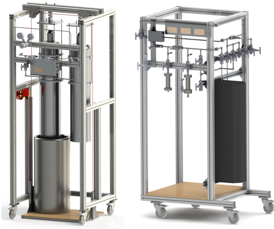
Figure 4.18. The gas-storage system (left) and the gas-recirculation system (right). [Hil14]
