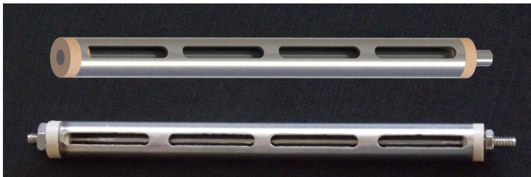
Figure 4.14. The levelmeter of the buffer volume. On top the rendered CAD-version, on bottom a photography. One can see the long holes for the liquid to enter and the PEEK-end caps.[Gro17]
