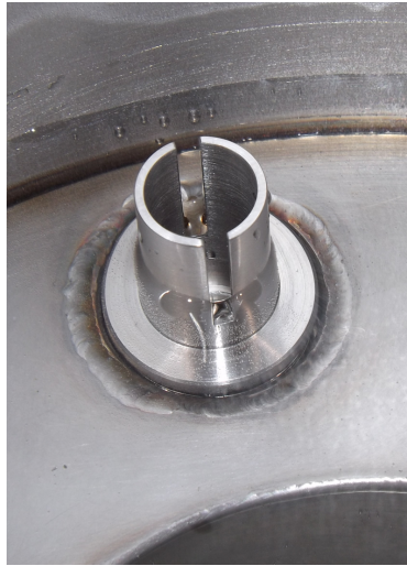
Figure 4.17. Photo of the leveling bellow in the TPC-vessel. The vessel is filled with water to test the surface tension effect on the gaps.
