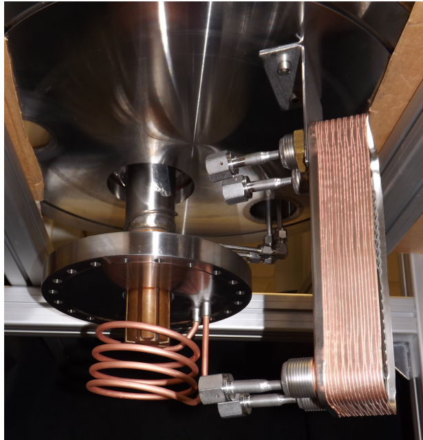
Figure 4.20. View into the cryostat of the cooling chamber. One can see the cold-finger of the PTR and the copper spiral for emergency and add-on cooling with liquid nitrogen. Copper spiral and cold finger are enclosed with a half-sphere from the bottom, serving as funnel for the liquefied xenon. On the right, one can see the heat exchanger we used. The heat exchanger was later mounted in the cryostat of the TPC. [Gro17]
