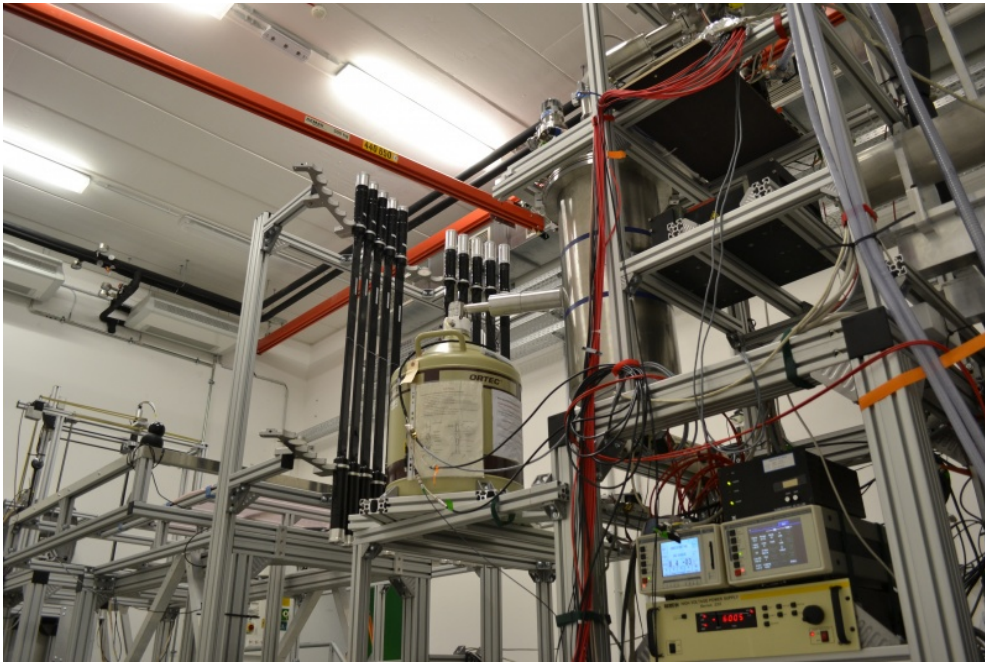
Figure 4.26. The Compton setup at HZDR. The germanium detector is mounted in front of the plastic scintillators. The collimator made from lead brick sits below the cooling chamber and in front of the neutron beam tube. Of course, for the neutron scattering experiment, germanium detector and collimator have been removed.[Gro17]
