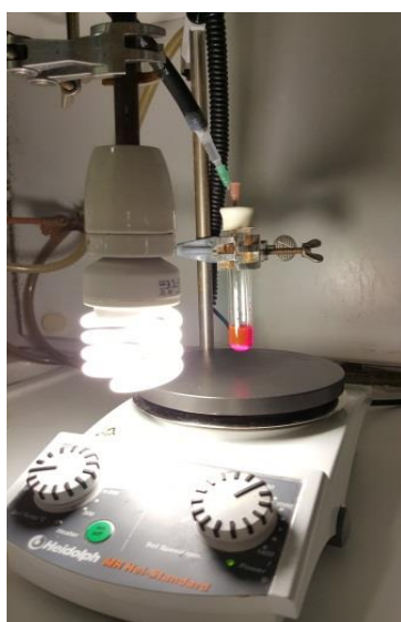
Figure 25. Typical reaction setup for the initial studies.
