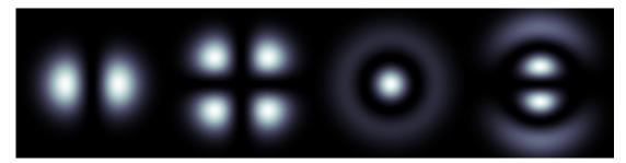
Figure 8.2: Examples of higher order modes in the Hermite-Gauss (left-hand side) and the Laguerre-Gauss (right-hand side) set of modes.
