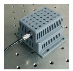
(b) Assembled climate board inside its housing.
