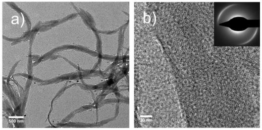
**Figure 3-11.** a) Electron microscopy of **3-1a** fibers grown from THF:MeOH=1:1 solution, b) HRTEM image of a fiber displaying columnar structures of **3-1a**, c) electron diffraction pattern with reflections assigned to the  $\pi$ -stacking distance of 0.35 nm.
