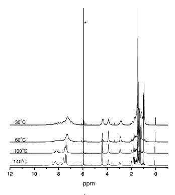
**Figure 3-5.** Temperature-dependant  $^1$ H NMR (500 MHz) spectra of **3-2b** in d-tetrachloroethane (\*)
