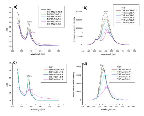
Figure 3-10. UV-vis and photoluminescence spectra for **3-1a** (a and b) and **3-1b** (c and d) in THF-MeOH mixed solvents  $(1.0 \times 10^{-5} \text{ M})$ .
