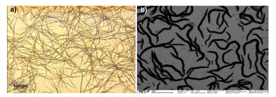
Figure 1-9. Self-assembly of HBCs into fibrous nanostructure on the surface.
