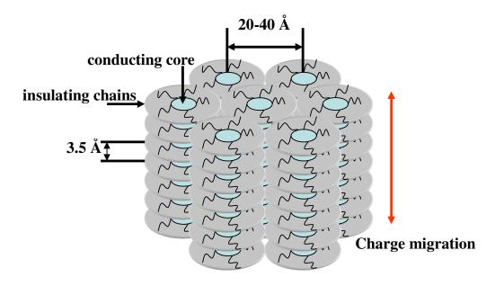
Figure 1-4. Schematic view of charge migration in columnar phase.
