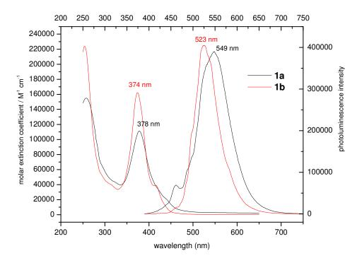
**Figure 3-6.** UV-vis and photoluminescence spectra for **3-1a** (black) and **3-1b** (red) in THF  $(5.0 \times 10^{-6} \text{M})$ .
