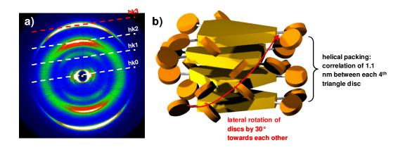
**Figure 4-7.** a) 2D-WAXS of an extruded fibre of **4-10** including the Miller's indices for the intracolumnar packing and b) schematic illustration of a helical pitch (the alkyl side chains are omitted for simplicity).
