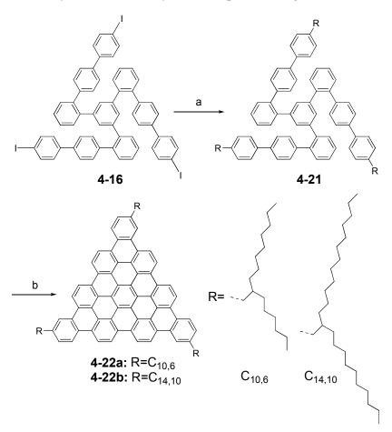
**Scheme 4-3.** Synthesis of triangle-shaped discotic graphenes **4-22**. a) RBrZn, Pd(dppf)Cl<sub>2</sub>, DMA, 50°C, 43% for **4-21a**, 30% for **4-21b**; b) FeCl<sub>3</sub>/CH<sub>3</sub>NO<sub>2</sub>, CH<sub>2</sub>Cl<sub>2</sub>, 89% for **4-22a**, 86% for **4-22b**. dppf: 1,1′-bis(diphenylphosphino)ferrocene; DMA: dimethylacetamide.
