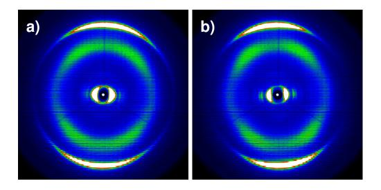
**Figure 3-9.** 2D-WAXS patterns of the corresponding alignment of the superstructures in the extruded filaments for a) **3-1b** and b) **3-2b**.
