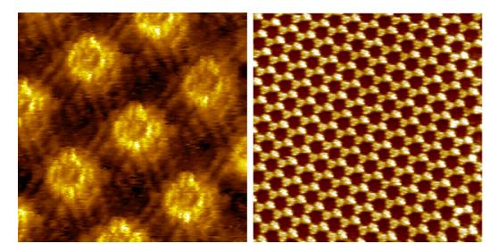
**Figure 1-8.** Self-assembly of hexadecyl-HBC (left) and triangle-shaped PAHs (right) on the liquid-solid interface.
