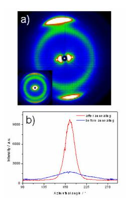
Figure 6-2. a) 2D-WAXS pattern of **4-22b** after annealing (inset shows before annealing), b) azimuthal integration of the meridional reflection related to the  $\pi$ -stacking.
