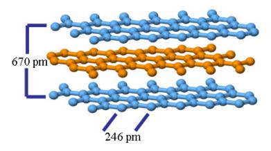
Figure 1-1. Layer structure of graphite.
