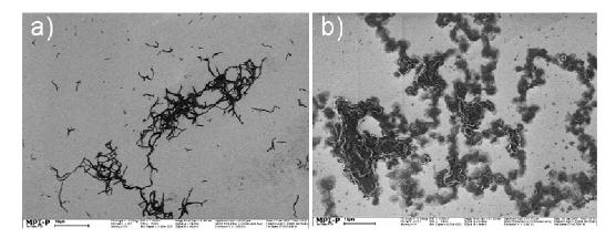
**Figure 3-12.** SEM pictures of **3-1a** (a) and **3-1b** (b) nanostructures grown from THF:MeOH = 1:1 solution.
