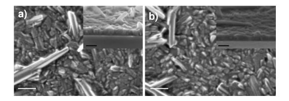
**Figure 4-18.** SEM images: top view images (scale bar for 100 nm) and cross-section view (inset, scale bar for 500 nm) of a) **4-22b**:PDI and b) **4-22a**:PDI (both in a ratio of 4:6). All the films were annealed at 120 °C for 1h.
