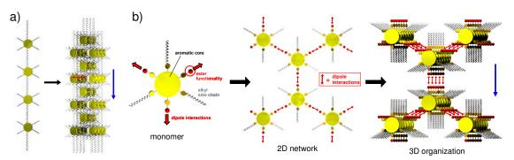
**Figure 3-8.** Schematic illustration of self-assembly and alignment orientation during mechanical processing of a) main chain discotic polymers (red arrow characterises  $\pi$ -stacking interactions), and b) compound **3-1a** which assembles first *via* dipole interactions into a 2D network and in a further step *via*  $\pi$ -stacking into a 3D hexagonal columnar organization. In both cases, the blue arrow indicates the alignment direction to which the columns are arranged perpendicularly.
