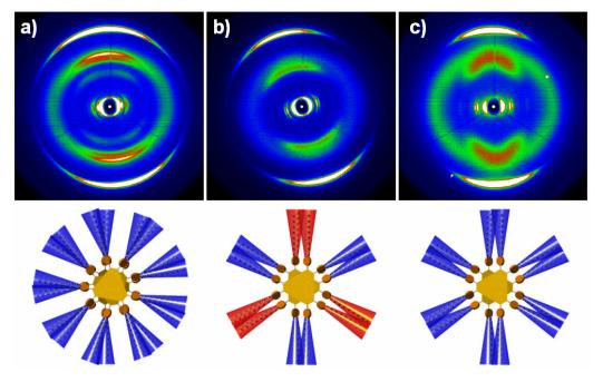
**Figure 5-11** 2D-WAXS patterns and corresponding schematic illustrations of top-viewed molecules stacked on top of each other, a) **4-10**, b) **5-9** (both patterns recorded at 30 °C) and c) **4-10** at 180 °C. Blue and red substituents indicate alkyl and glycol chains respectively.
