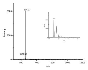
**Figure.2-4.** MALDI-TOF mass spectrum of compound **2-7** (the peak at 620.66 is ascribed to the scissor of *tert*-butyl group by MALDI-TOF spectrometer)
