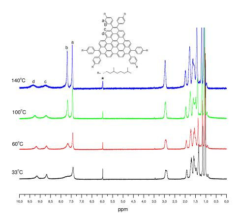
**Figure 4-6.** Temperature-dependent <sup>1</sup>H NMR (500 MHz) spectra of **4-10** in [D<sub>2</sub>]tetrachloroethane(\*).
