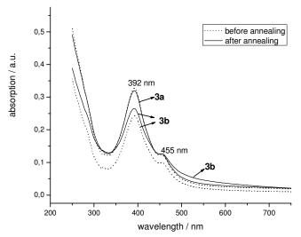
**Figure 4-14.** UV-vis absorption spectra of **4-22a** and **4-22b** in thin films (thickness of  $100 \pm 10$  nm) before (dotted line) and after annealing at  $120^{\circ}$ C (solid line).
