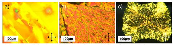
**Figure 5-6.** Polarized optical microscopy images of **5-1b** cooled from the isotropic phase by a) 0.1 °C/min, b) 1 °C/min and c) 10 °C/min.
