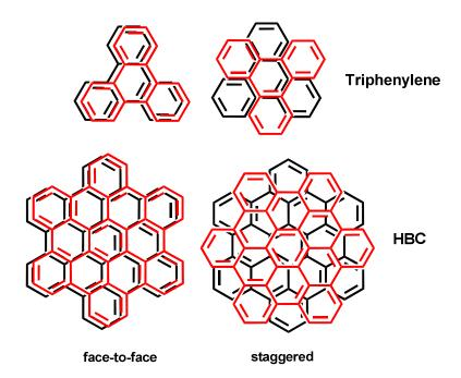
**Chart 5-1.** Illustration of the face-to-face and staggered stacking of two typical discotic molecules: triphenylene (staggered twisting angle is 60°); HBC (staggered twisting angle is 30°).
