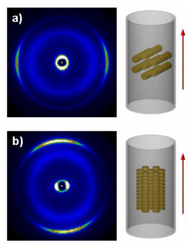
**Figure 3-7.** 2D-WAXS patterns and schematic illustration of the corresponding alignment of the columnar superstructures in the extruded filaments (red arrow indicates the extrusion direction) for a) **3-1a** and b) **3-2a**.
