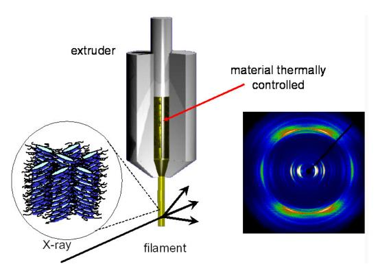
**Figure 1-7.** Schematic illustration of the experimental set up and principle for 2D-WAXS measurements on extruded filaments.
