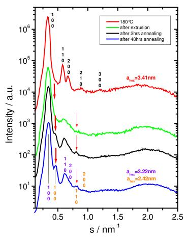
**Figure 4-8:** Scattering intensity as a function of the scattering vector of **4-10**. The experiments after annealing were performed at 30 °C.
