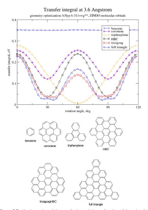
**Figure 5-7.** Absolute value of the transfer integral J as a function of the azimuthal rotation angle.
