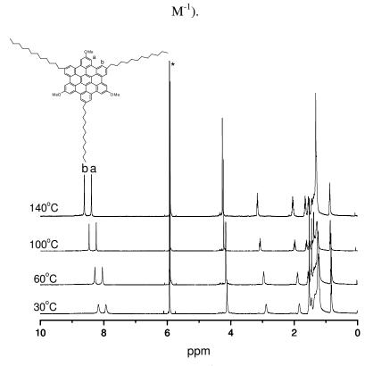
**Figure 3-16.** Temperature dependent <sup>1</sup>H NMR spectra of **3-16b** in  $d^2$ -1,1,2,2-tetrachloroethane (2.38 × 10<sup>-3</sup> M).
