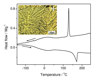
**Figure 2-5.** DSC traces of **2-14** during the first cooling and the second heating cycle at 10 °C/min; inset displays an image from polarized optical microscopy (POM) at cross-polarizers after cooling from the isotropic phase at 1 °C/min.
