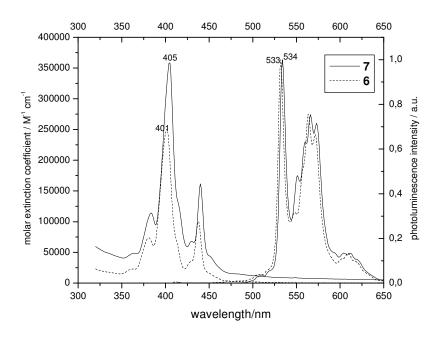
**Figure 4-5.** UV-vis and photoluminescence spectra of **4-6** and **4-7**  $(1.0 \times 10^{-6} \,\mathrm{M})$  in 1,2,4-trichlorobenzene). Dashed line: **4-6**, black line: **4-7**.
