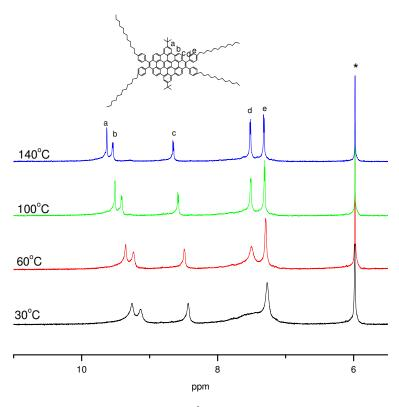
**Figure 5-2.** Temperature-dependant  $^{1}$ H NMR (500MHz) spectra of **5-1b** in d-CD<sub>2</sub>Cl<sub>2</sub>CD<sub>2</sub>Cl<sub>2</sub>.
