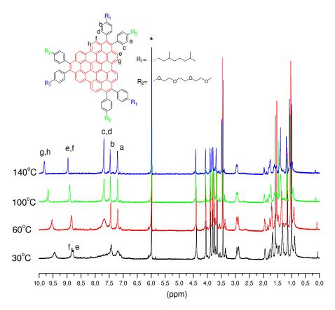
**Figure 5-10.** Temperature-dependent <sup>1</sup>H NMR (700 MHz) spectra of **5-9** in [D<sub>2</sub>]tetrachloroethane(\*).
