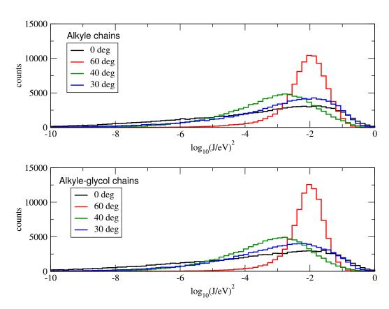
**Figure 5-15.** Distribution functions of the transfer integrals for two different systems and four different initial twist angles. Up (**4-10**) and down (**5-9**).
