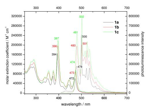
**Figure 5-1.** UV-vis and photoluminescence spectra of **5-1a** (black), **5-1b** (red) and **5-1c** (green)  $(1.0 \times 10^{-6} \text{M in CHCl}_3)$ .
