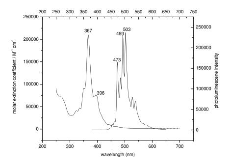
Figure 3-15. UV-vis and photoluminescence spectra of 3-16b in CHCl<sub>3</sub> (1.0×10<sup>-6</sup>
