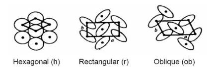
**Figure 1-3.** Top view of two-dimensional lattices of columnar phases. The ellipses denote discs that are tilted with respect to the columnar axis.
