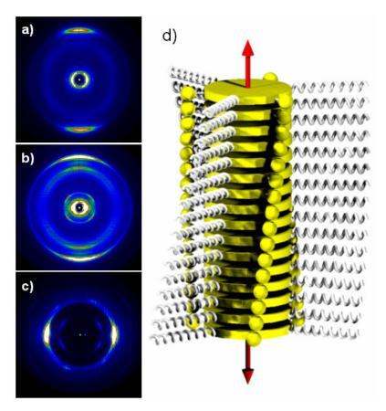
**Figure 3-17**. Structural characterization of **3-16b**; a) 2D-WAXS at 170 °C and b) at 30 °C after annealing; c) 2D-SAXS at 30 °C after annealing; d) schematic illustration of the intracolumnar arrangement of **3-16b** at 30 °C into a helical organization with a disc rotation of *ca* 2.14°.
