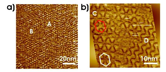
**Figure 2-10.** a) STM current image of molecules **2-14**, the "zigzag" structure marked by A, and the dimer structure by B. b) STM height image of molecules **2-15**, the flowerlike pattern in C domain, the zigzag in D domain.
