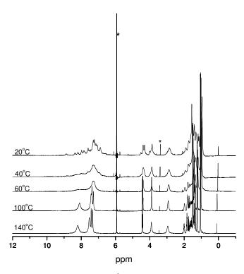
**Figure 3-4.** Temperature-dependant  $^{1}$ H NMR (500 MHz) spectra of **3-1b** in d-tetrachloroethane (\*)
