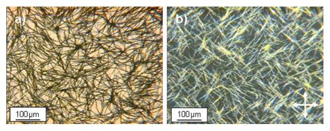
**Figure 3-18.** Optical images of the morphology of **3-16b** drop-cast from o-dichlorobenzene (1.0 × 10<sup>-4</sup> M) in a) without and b) with cross-polarizers.
