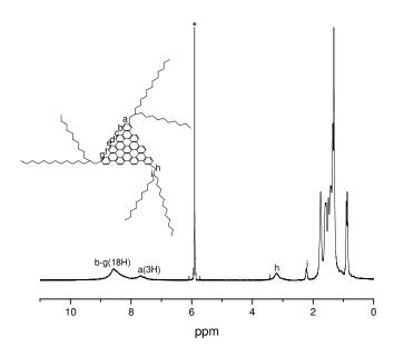
Figure 4-12. <sup>1</sup>H NMR spectrum of 4-22a at 140°C in CDCl<sub>2</sub>CDCl<sub>2</sub> (\*).
