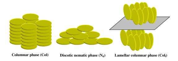
Figure 1-2. Schematic representation of different mesophases of DLCs.
