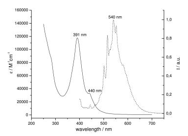
**Figure 4-13.** UV-vis absorption (solid line,  $1.0 \times 10^{-6}$  M) and fluorescence (dashed line,  $1.0 \times 10^{-7}$  M) spectra of **4-22b** in CHCl<sub>3</sub>.
