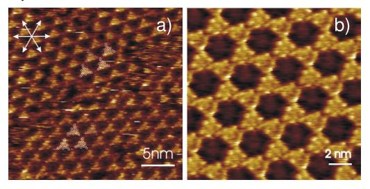
Figure 4-9. STM current images of a) 4-4 and b) 4-10 at the HOPG-solution.
