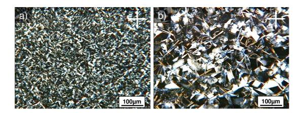
**Figure 2-8.** POM images with cross-polarizers of **2-15** cooled from the isotropic phase by a) 1 °C/min and b) 0.1 °C/min.
