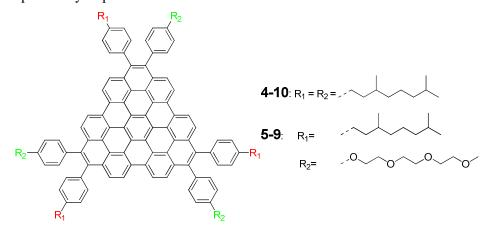
**Figure 5-8.** Structures of studied triangle-shaped discotics.
