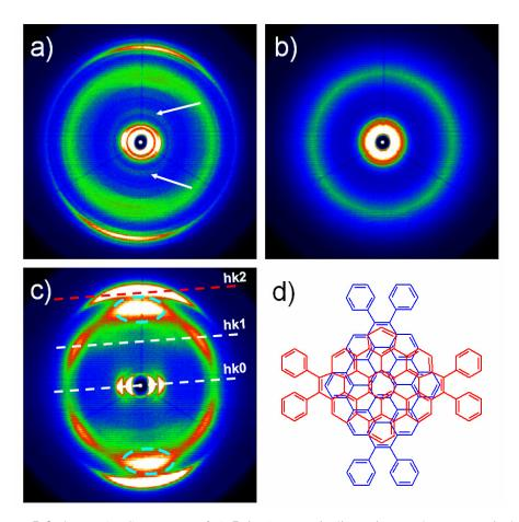
**Figure 5-3.** 2D-WAXS patterns of a) **5-1a** (arrows indicate intracolumnar periods of 1 nm), b) **5-1b**, c) **5-1c** (Miller's indices for the intracolumnar stacking and the higher order reflections are indicated) and d) illustration of the rotation assigned for **5-1c**.
