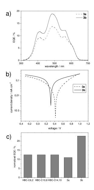
**Figure 4-17.** a) *EQE* plots for ITO/ **4-22b**(solid line) and **4-22a** (dotted line):PDI (4:6)/ Ag device; b) corresponding I –V characteristics under one sun illumination at 490 nm; c) normalized *EQE* by the chromophore density for previously reported swallow-tailed HBCs<sup>[24b]</sup> and compounds **4-22**. The chromophore density was determined by ratio between the number of carbon atoms of the aromatic core and the side chains.
