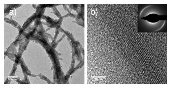
**Figure 3-13.** a) Electron microscopy of **3-1b** fibers grown from THF:MeOH=1:1 solution, b) HRTEM image of a fiber displaying columnar structures of **3-1b**, electron diffraction pattern with reflections (inset) assigned to the  $\pi$ -stacking distance of 0.35 nm.
