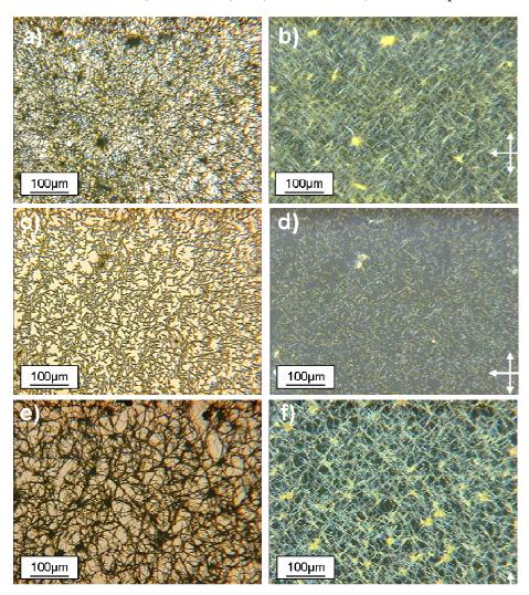
**Figure 3-19**. Optical images of the morphology of **1b** drop-cast from toluene (a and b), CHCl<sub>3</sub> (c and d), and THF (e and f) solution  $(1.0 \times 10^{-4} \, \text{M})$  without and with cross-polarizers.
