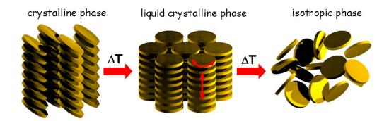
**Figure 1-6.** Schematic representation of the self-organization within three phases of substituted HBCs.
