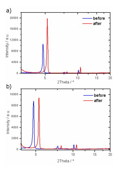
**Figure 4-16.** Thin film diffraction of ) **4-22b** and b) **4-22a** before and after annealing of spin-coated layers. For comparisons, the diffractorgram before annealing (blue plot) is shifted by 0.5° to lower angles.
