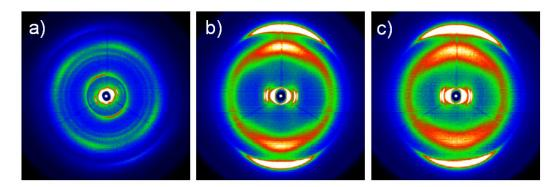
**Figure 5-4.** 2D-WAXS patterns of a) **5-1a** at 180 °C, and **5-1c** at b) 30 °C and c) at 160 °C.
