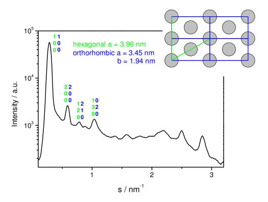
**Figure 2-7.** Equatorial integration of the 2D pattern of **2-14** plotted as the scattering intensity as a function of the scattering vector s. The reflections are assigned by the Miller's indices indicating two different unit cells, hexagonal and orthorhombic. The corresponding intercolumnar arrangement of **2-14** is illustrated in the inset.
