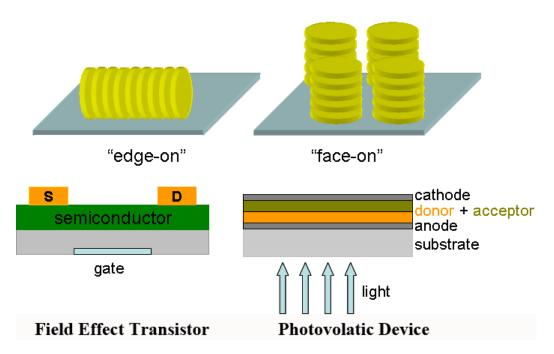
**Figure 1-10.** Schematic representation of two different electronic device types and their desired arrangement of discotics as electronic materials.
