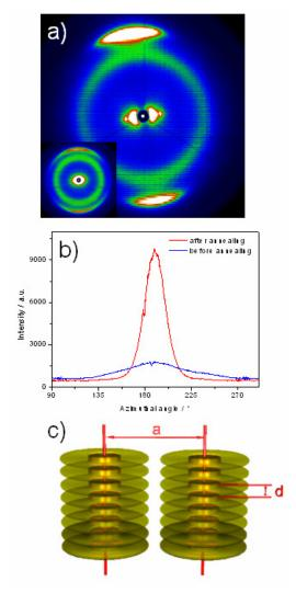
**Figure 4-15.** a) 2D-WAXS pattern of **4-22b** after annealing (inset shows before annealing), b) azimuthal integration of the meridional reflection related to the  $\pi$ -stacking, c) schematic illustration of the columnar organization of **4-22a** and **4-22b**.
