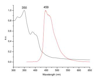
**Figure 4-3**. UV-visible absorption and photoluminescence spectra of 4-4 (in CHCl<sub>2</sub>CHCl<sub>2</sub>)
