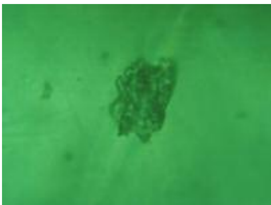
Figure 18a: Talc flakes usually are very small aggregates in Santa Terezinha emerald, the big one as shown in photo is very infrequent. x50
