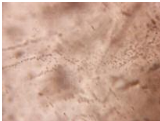
Figure 47: Tiny particles (fluid inclusions) in Uralian emeralds resembling those in emeralds from Capoeirana. x50
