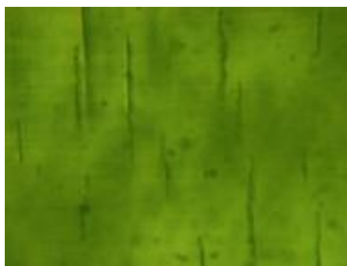
Figure 20: Fissure system parallel to the c axis in emeralds from Socoto. x10
