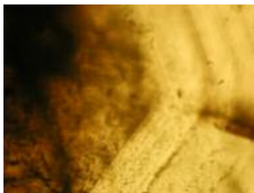
Figure 22: The dark brown core zone is caused by the conglomeration of mica and some carbonate minerals. x50
