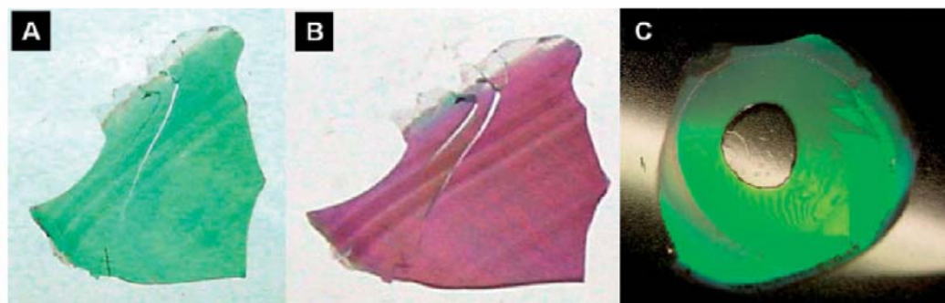
Figure 2. OC1 inverse opal: A) free standing film, top view, B) free standing film, tilted viewing angle, and C) OC1 replica on a glass substrate (2 cm × 2 cm) (the sample for A and B was fabricated by J. Ye [26] ).
