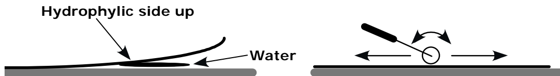
Figure 2: Assembling glass plate with Gel Bond PAG film
