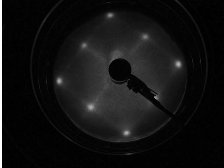
Figure 4.20: LEED diffraction pattern for a \text{Co}_2\text{Cr}_{0.6}\text{Fe}_{0.4}\text{Al} film deposited on Fe buffer layer and annealed at 550^\circ\text{C} for 5 min. The energy of the electron is 120 eV.
