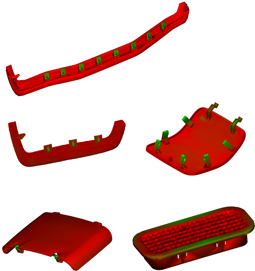
Fig. 43: The results of phase II. Vertices with a large displacement are marked in green and vertices with a small displacement in red.
