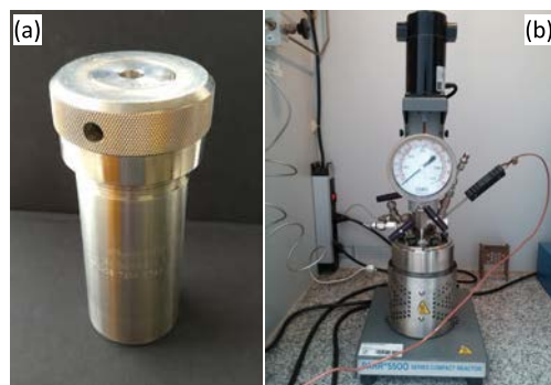
Figure 2.6. Reactors for solvothermal processing: (a) solvothermal bomb and (b) autoclave reactor with gas inlet and temperature–pressure monitoring.
