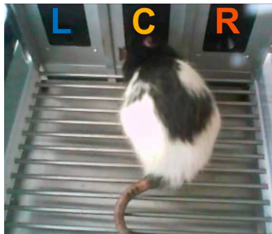
Figure 1. Picture of the operant chamber with a rat poking into the center (reward) port. Reward (30 \mu L of water) could be triggered by poking into the left (L) and right (R) ports at random intervals. Water reward is delivered at the center (C) port. The stainless steel grid floor was used to deliver mild foot shocks in later experiments.
