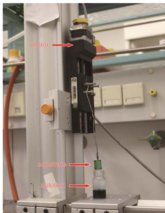
Figure 9.3 Photograph of dip-coating setup.
