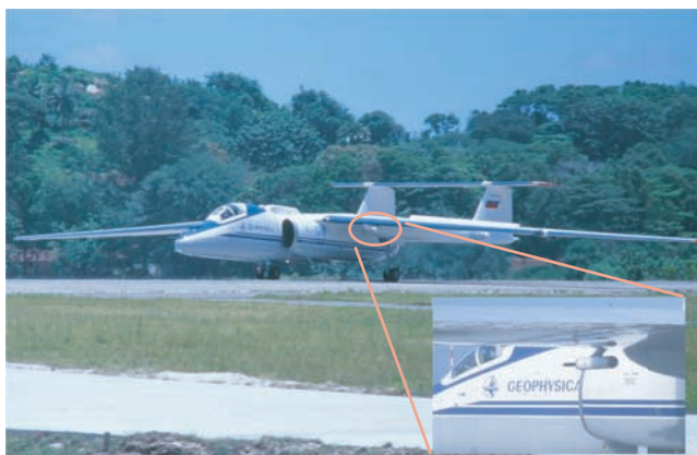
Figure 1. The Russian high-altitude research aircraft “Geophysica” before takeoff on the airport of Mahé, Seychelles. The mounting of the FSSP-300 sonde underneath the left wing is shown in the small photo.
