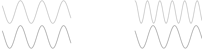
Figure 5.4: Schematic geometric interpretation of commensurability. Two bare commensurate walls (left) can lock, whereas bare incommensurate surfaces (right) cannot lock if the lattice constants are (sufficiently) different.
