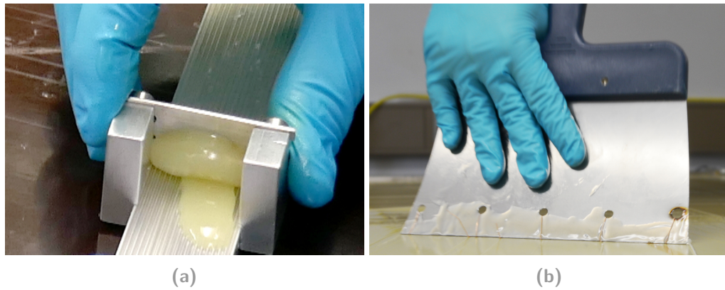
Figure 4.24. Gluing tools used during the construction. A spill of the glue over the sides of the aluminum bars is avoided by the dedicated gluing tool (a). The thickness of the glue layer on the FR4 boards is fixed by wires, bend over the edge of a spatula (b).
