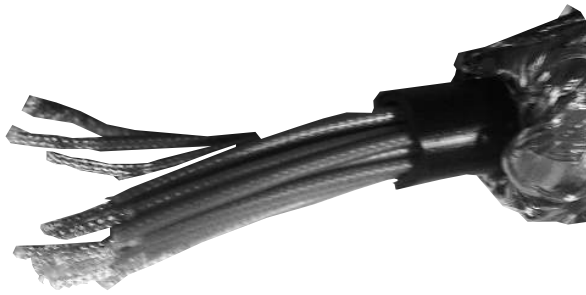
Fig. D.10 Bundle of 16 RG178 cables inside the insulation tube and shielding
