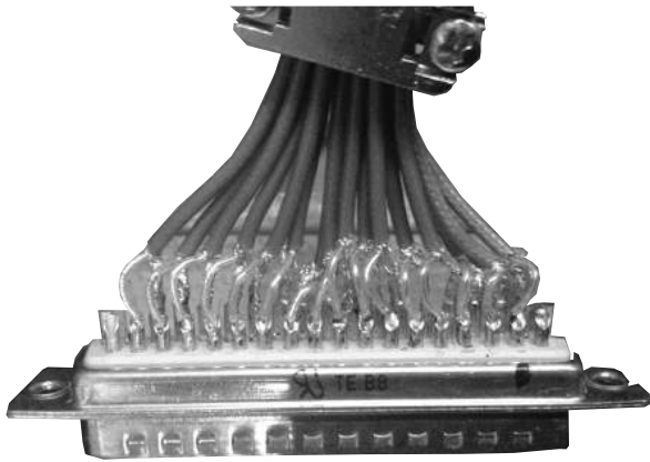
Fig. D.12 Image of dedicated GND pins for each channels
