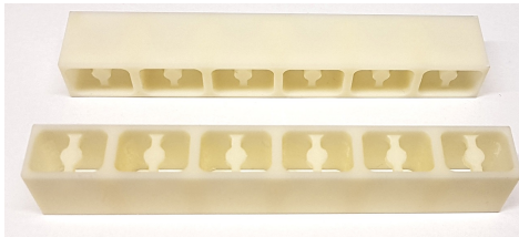
(b) Diffuser components. Basic dimensions of each part are 120 mm × 15 mm × 20 mm.
