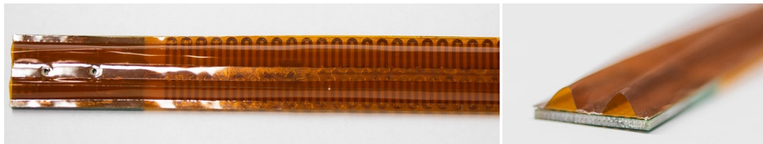
Figure 9.16.: Heatable strip prototype with v-folds.
