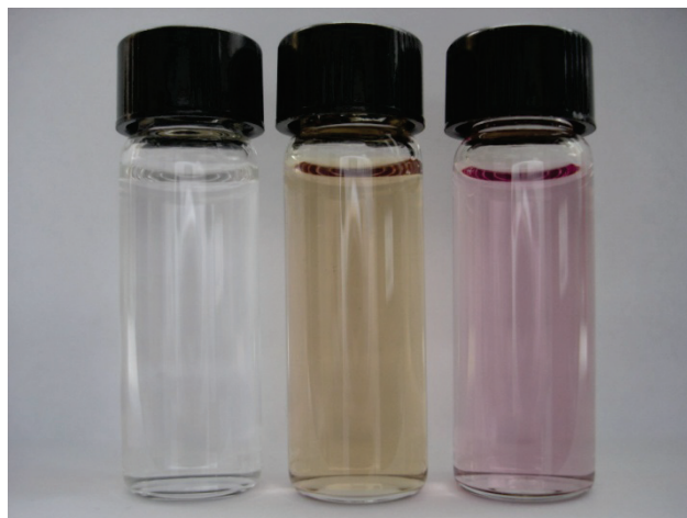
Figure 5.1: Photograph demonstrating color shifts in water. Left: NaPSS brush ( c(\text{NaPSS}) = 240 \mu\text{M} ), center: NaPSS brush with TAPP ( c(\text{NaPSS}) = 240 \mu\text{M} , c(\text{TAPP}) = 25 \mu\text{M} , l = 0.4 ), right: TAPP ( c(\text{TAPP}) = 25 \mu\text{M} ).
