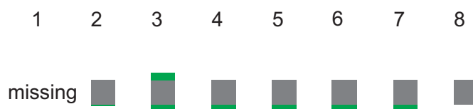
Fig. 3.25: Schematic representation of PMMA film location on each side of the individual cantilever (array OS-S 500 #042). Cantilever 1 broke during the synthesis.
