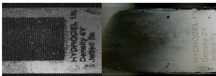
Fig. 3.5: Hydrogel from an 1% aqueous polymer solution deposited by an inkjet printer. With Dave Tune, 9D Tech.
