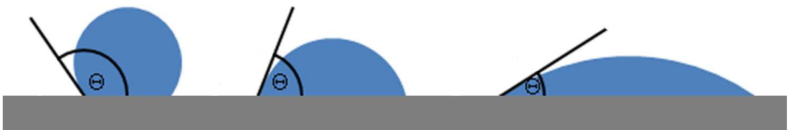
Fig. 2.1: Contact angle of a water droplet on an ultrahydrophobic (left), hydrophobic (center) and very hydrophilic (right) surface.
