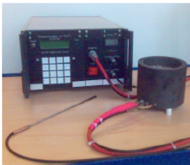
Figure 3.6 The home-built metal bath heater and temperature control equipped with two Pt100 thermocouples. One is situated inside the brass heater. The second one is introduced in a thin glass tube and placed into the flask measuring the actual reaction temperature. The unit is connected to a computer, which records the temperature read-out of both thermometers.
