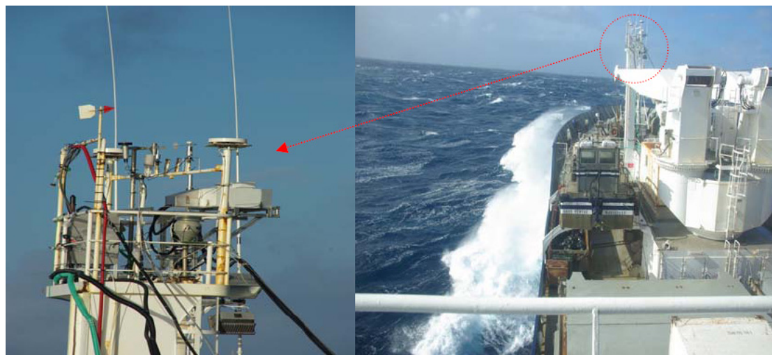
Figure 2.3 The position and setup of the inlet line on the atmospheric mast during the MD 160 cruise.
