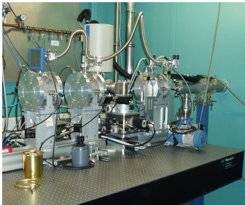
Fig. 3.13. Fluorescence set-up in use in the experimental hutch at the INE-Beamline.
