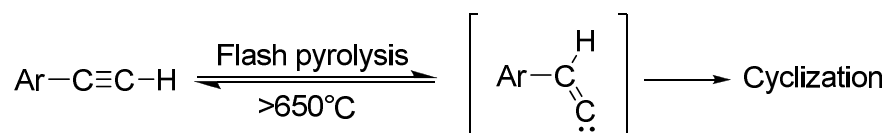
Figure 1-2. The reversible rearrangement of terminal acetylenes to vinylidenes.
