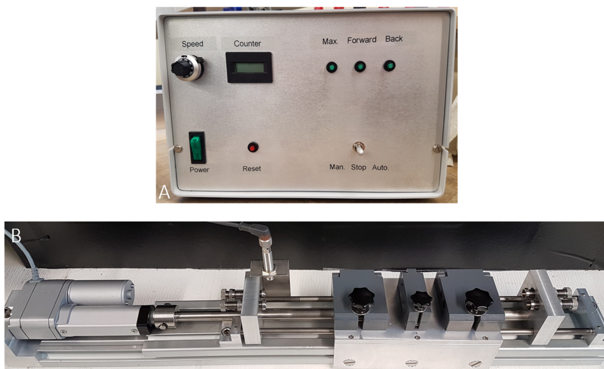
Figure S2. Custom-built, automatic extrusion device (B) with separate control unit (A).
