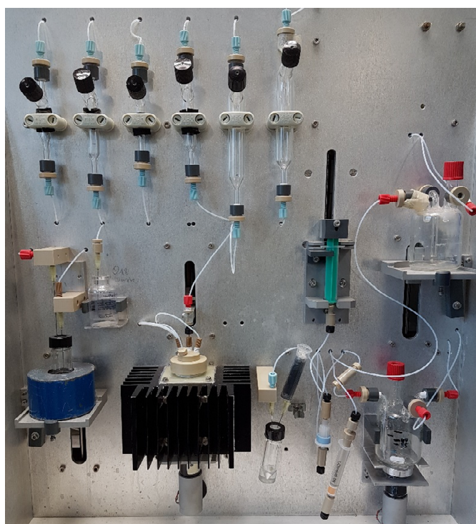
Figure S-6. Front panel of the semi-automatic custom modular system used for the synthesis of [ 18 F]F-TEG-N 3 .
