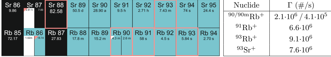
Figure 4.24: Left: Excerpt of the Karlsruhe nuclide chart, showing the investigated species and their half-lives, respectively the natural abundance of stable nuclides. Right: Fission yield of the determined species, produced within the used ^{235}\text{U} -target.
