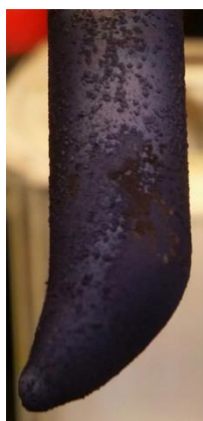
Figure S1. Photograph of Au(TPP) sublimed onto the cold finger of the sublimation apparatus.
