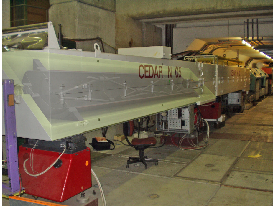
Figure 3.1: Picture of CEDAR detector in the M2 beam line overlaid by an illustrated cut through the detector. The high pressure vessel containing helium was covered by an insulation box to shield the vessel against thermal and physical influences.
