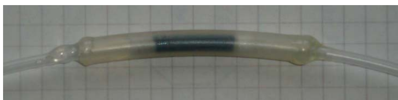
Figure 35: Photo of a charcoal trap. Picture taken from [118]
